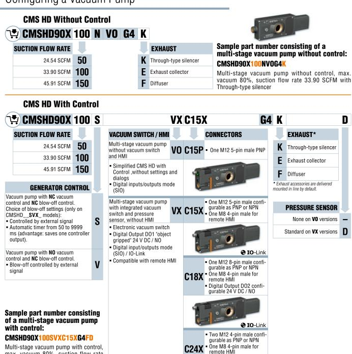
max. vacuum 80%, suction flow rate 33.90 SCFM, NC vacuum and blow-off control, one M12 5-pin connector and one M8 4-pin connector, with diffuser
