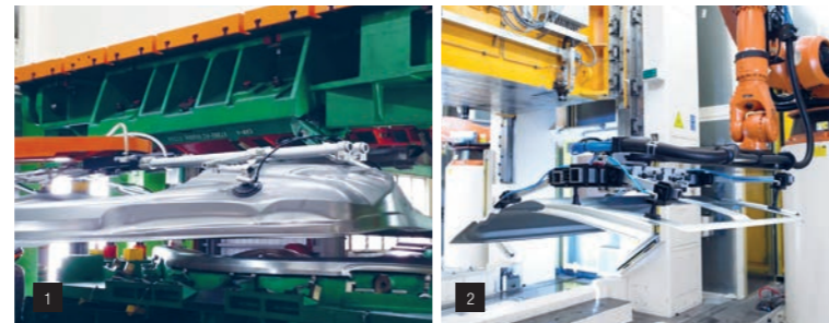
1 2 LEMAX+ vacuum pumps and C-series high-performance suction cups for handling stamped parts.
